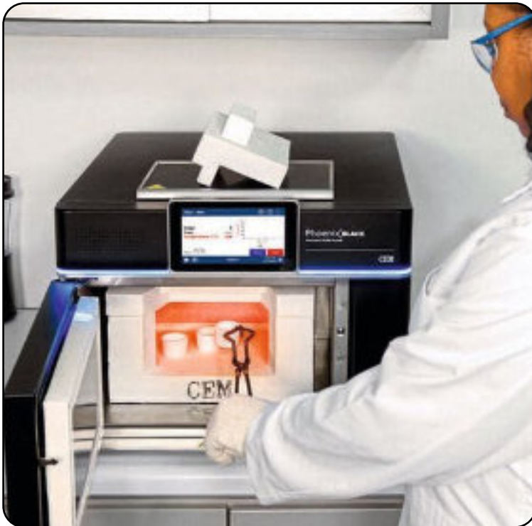
;- Muffle Furnace Test is used for PVC pipes to verify material composition and thermal stability by measuring residue content under high temperatures, ensuring consistent quality and compliance with required standards.
